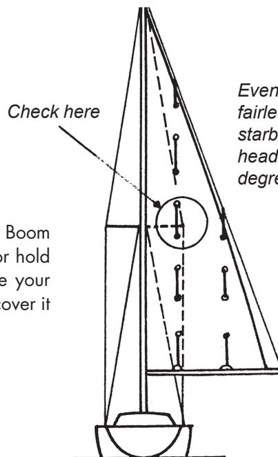
*Even number of fairleads, tabs on the starboards side, head boat to port 5 degrees*
